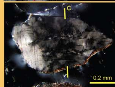
Figure 7 (above) – Polarized-light photomicrograph showing multiple sets of unusually well-developed, variably decorated PDFs (P2 planes) within polycrystalline quartz grain, Buck Ridge Road sample.
