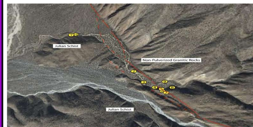
Location of samples 1 through 10 for the White Wash pulverized granite locality. On the southwest side of the fault, the granite occurs as dike rock emplaced into Julian Schist (factually a gneissic schist in this area). The granitic rock is pulverized whereas the schist is mostly just fractured.
