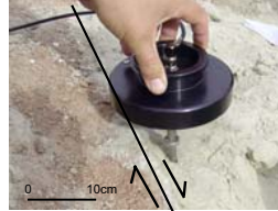
Figure 5. Close up of Figure 5 showing the placement of the TDR ground probe adjacent to the NW striking dextral fault.
