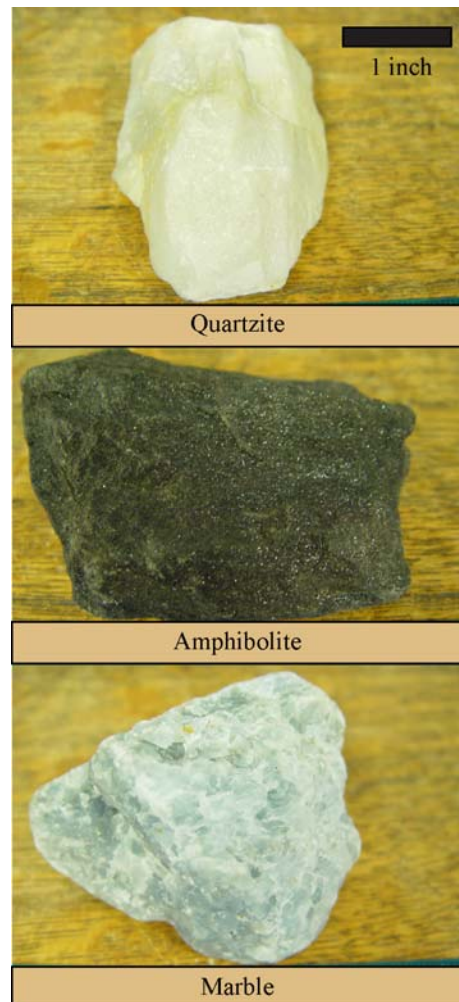
Figure 6. Nonfoliated varieties of metamorphic rocks include quartzite, amphibolite, and marble. The protoliths of these include quartz arenite (or chert), basalt, and limestone.
