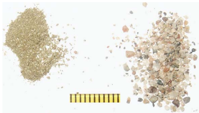
Figure 5. Mud versus sand. The pile of sediment on the left includes mostly mud-sized particles while the pile on the right is composed of sand-sized material. The smallest increment shown on the scale is 1 mm.
